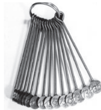
Fig. 49: Example of radius gauges (own production)
