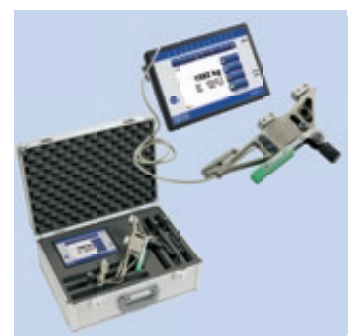
Fig. 38: Simultaneous measurement of rope tensile force
