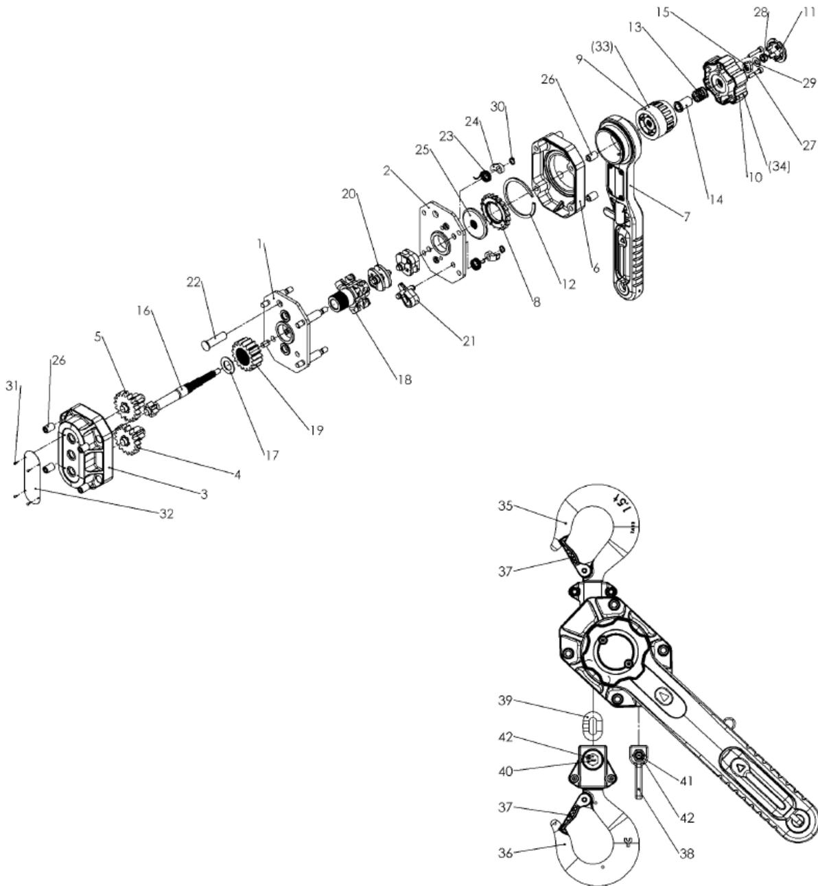
**Hebelzug ERGO 360° 1500 kg****Lever hoist ERGO 360° 1500 kg**
