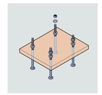
Check the anchor position and protrusions after concreting according to the respective layout specification. Maximum tolerances are to be taken from the below table.
