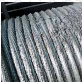
Typical structural damages on ropes in crossover sections of multi-layer winches.
