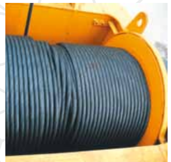
Incorrect spooling can reduce the lifetime of the rope considerably! Improvement of spooling behaviour is possible and achievable – with our support.
