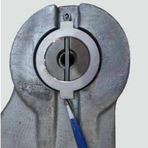
Fig. 8.2.4.4: Inserting and fixing the pin
