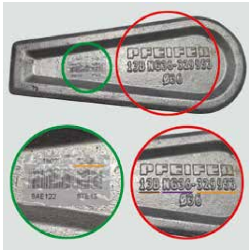
Fig. 6.3.2.1: Marking of the wedge
